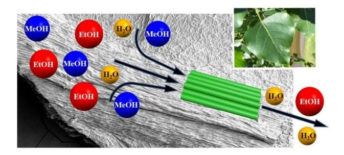
Micrograph photo (total width approximately 1,5 mm) showing the novel adsorbent material that was produced using a poplar leave as a template. The channel architecture is clearly noticeable. The drawings show the tubular structure (green) and the molecular separation process. Credit: HIMS
