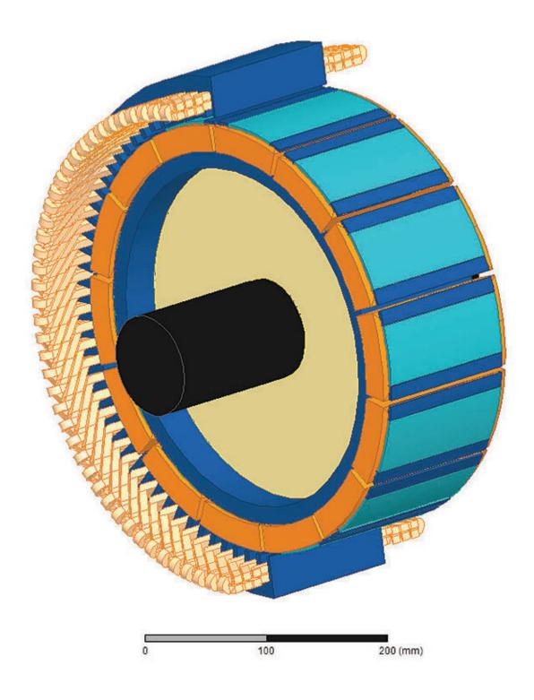
Purdue University researchers developed a parallel inner-magnet device to reduce the size and increase the efficiency of the moderate- to low-power electric generators. Credit: Purdue University
