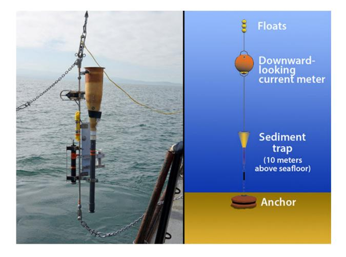
As part of the Coordinated Canyon Experiment, geologists used sediment traps to collect sediments carried down Monterey Canyon. Credit: MBARI
