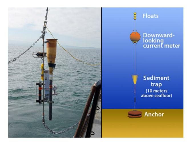
As part of the Coordinated Canyon Experiment, geologists used sediment traps to collect sediments carried down Monterey Canyon. Credit: MBARI
