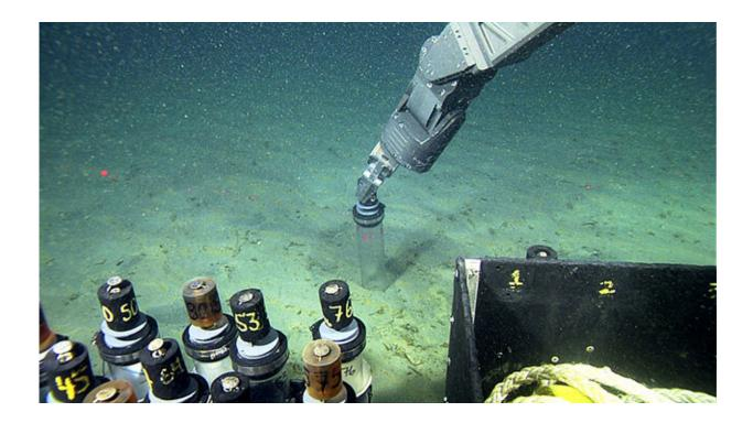
During the Coordinated Canyon Experiment, researchers collected hundreds of sediment samples from the floor of Monterey Canyon using underwater robots and "push cores" (the clear plastic tube being inserted into the sediment). Credit: MBARI
