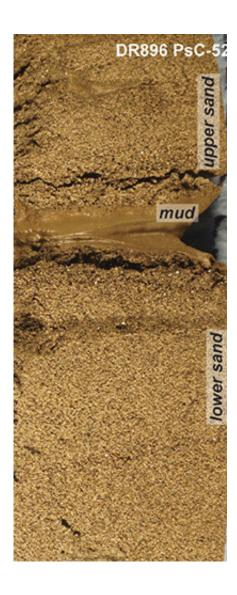
This photograph shows a cross section of sediment collected in a push core from Monterey Canyon. Most of the sediment is relatively uniform sand. Credit: MBARI
