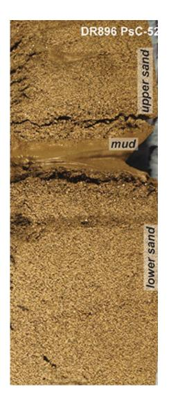
This photograph shows a cross section of sediment collected in a push core from Monterey Canyon. Most of the sediment is relatively uniform sand. Credit: MBARI
