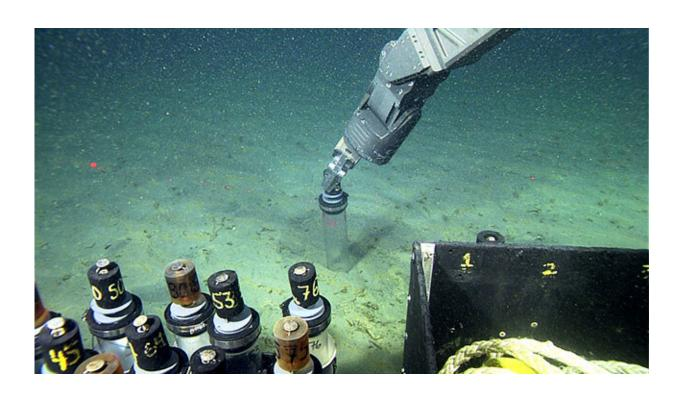
During the Coordinated Canyon Experiment, researchers collected hundreds of sediment samples from the floor of Monterey Canyon using underwater robots and "push cores" (the clear plastic tube being inserted into the sediment). Credit: MBARI
