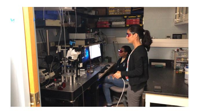
The instrument is designed to analyze the quality of liquids using the photoacoustic effect, or the generation of sound waves after light is absorbed in a material. The MU scientists believe this might be the first use of this technology to analyze such small liquid samples. Credit: University of Missouri
