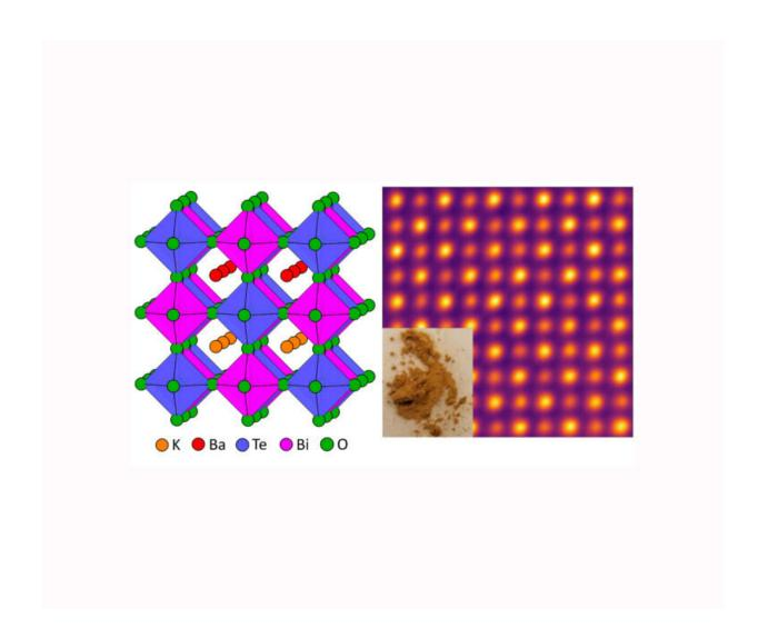
An atomic model of KBaTeBiO6 (left), the most promising of 30,000 oxides in a potential solar panel. At right is a scanning transmission electron micrograph
