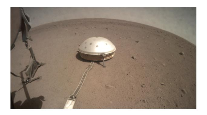
On June 28, 2019, NASA's InSight lander used its robotic arm to move the support structure for its digging instrument, informally called the "mole." This view was captured by the fisheye Instrument Context Camera under the lander's deck. Credit: NASA/JPL-Caltech
