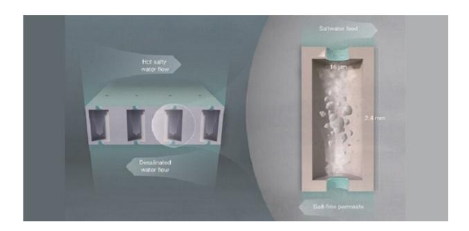
The membrane's pores entrap air upon immersion in water, separating the liquids on either side and allowing the transport of only pure water vapour from the hot to the cold side. Credit: Ivan Gromicho
