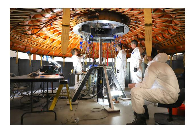
Engineers prepare for the flexible heat shield installation on the inflatable structure. The view is from bottom side, heat shield is on top. The gold straps hanging from the black triangles will be attached to the inflatable structure strapping and tensioned. Credit: NASA's Langley Research Center
