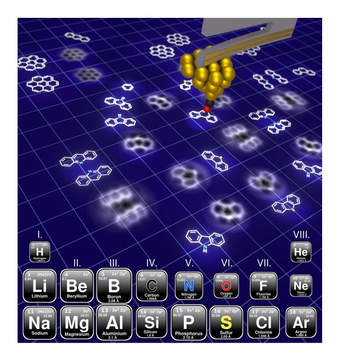
An illustration showing how nc-AFM can distinguish sulfur- and nitrogen-containing molecules commonly found in petroleum. A tuning fork (grey arm) with a highly sensitive tip containing a single carbon monoxide molecule (black is carbon and red is oxygen) is brought very close to the surface (outlined in white), with the oxygen molecule lying flat on the surface without making contact. As the tip scans across the surface, it "feels" the forces from the bonds
