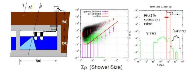
The China-Japan collaboration placed new water Cherenkov-type muon detectors under the existing cosmic-ray air-shower array in 2014. These underground muon detectors can suppress 99.92% of cosmic-ray background noise. Credit: IHEP
