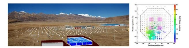
The left figure shows the Tibet ASgamma experiment (Tibet-III array+ Muon Detector array); The right figure shows an event display of the observed 449TeV photon-like air shower. Credit: IHEP
