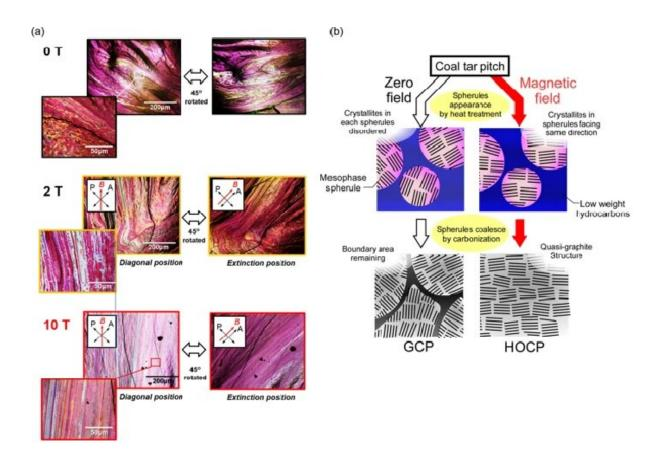
(a) Polarizing microscopy image of carbonized coal tar pitch prepared in the absence and presence of magnetic fields of 2?T and 10?T. All figures show the diagonal position and extinction position. (b) Schematic drawing of a magnetic field effect on the carbonization process of coal tar pitch. Credit: Springer Nature, Licensed under CC BY 4.0
