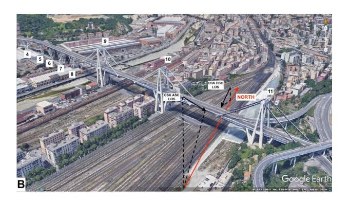
The Morandi Bridge before its collapse. New satellite radar imaging can show the movement of structures with millimetre accuracy. Credit: *Remote Sensing*
