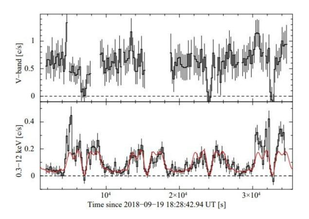
OM V-band (upper panel) and PN 0.3–12 keV (lower panel) background subtracted light curves of 2PBC J0658.0-1746 binned at 200 s, where for plotting purposes is also shown the result of a fit made with 7 sinusoids, the orbital period (8,565 s) and its first six harmonics (red curve). Image credit: Bernardini et al., 2019.
