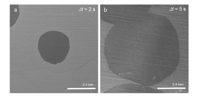
SEM images of graphene domains growing. They showed that 2 seconds was enough for a domain to grow to  $\sim 400~\mu m$  and that  $\sim 1~mm$  domains were formed after 5 seconds. The statistical growth rate is more than three orders of magnitude faster than typical graphene growth and three times faster than the
