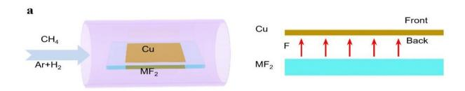
Schematic diagrams of the experimental design for locally introducing fluorine for graphene growth. Credit: IBS
