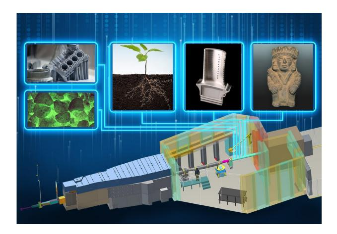
Artistic rendering of the VENUS imaging beamline under construction at ORNL's Spallation Neutron Source. VENUS will provide impactful insights into research areas such as those featured, including nuclear fuels such as uranium (left), additively manufactured materials, biological processes, engineered components, studies of archeological and natural materials. Credit: ORNL/Jill Hemman
