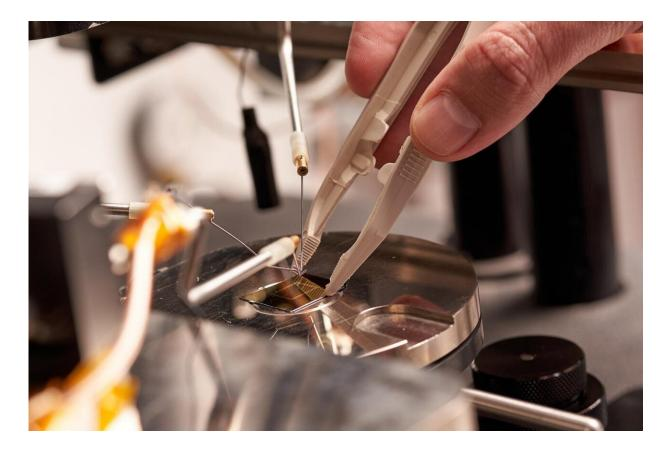
The brain-mimicking electronic chip uses light to create and modify memories. Credit: RMIT University
