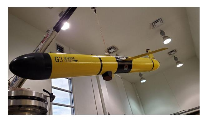
This autonomous glider, part of the University of South Florida glider fleet, is modified with sonar technology and will collect up close and personal data on the migrating animals in the water column. Credit: John Horne, University of Washington
