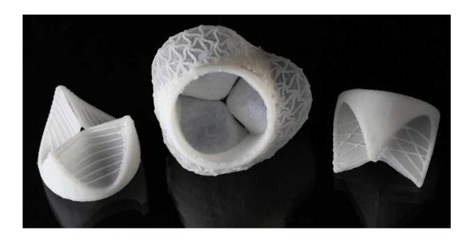
Multi-material additive manufacturing of patient-specific shaped heart valves. Elastomeric printing enables mechanical matching with the host biological tissue. Credit: Fergal Coulter / ETH Zurich
