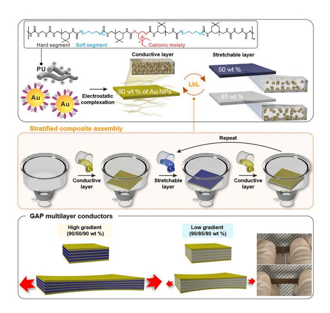
Stratified assembly of stretchable nanocomposites with different concentrations
