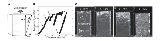
In situ TEM compression test showing that dislocation slip is responsible for the plastic deformation of an Mg single-crystal pillar under c-axis compression. (A) Hexagonal unit cell showing the loading orientation. (B) Stress-strain curve. (C) Snapshots showing an increase in dislocation density during compression. The dark-field TEM observation is conducted under a two-beam condition. Credit: *Science* (2019). DOI: 10.1126/science.aaw2843
