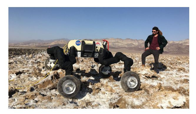
RoboSimian can walk on four legs, crawl, move like an inchworm and slide on its belly. In this photo it stands on the Devil's Golf Course in Death Valley, California, for field testing with engineer Brendan Chamberlain-Simon. Credit: NASA/JPL-Caltech
