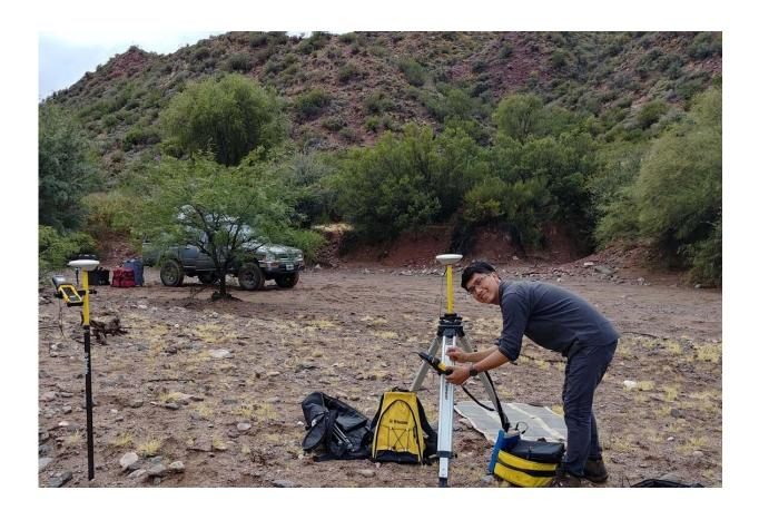
U of T's Jeremy Rimando sets up Differential Global Positioning System (DGPS) survey equipment to measure the amount of displacement on the Las Chacras Fault in San Juan, Argentina. Credit: Cesar Distante
