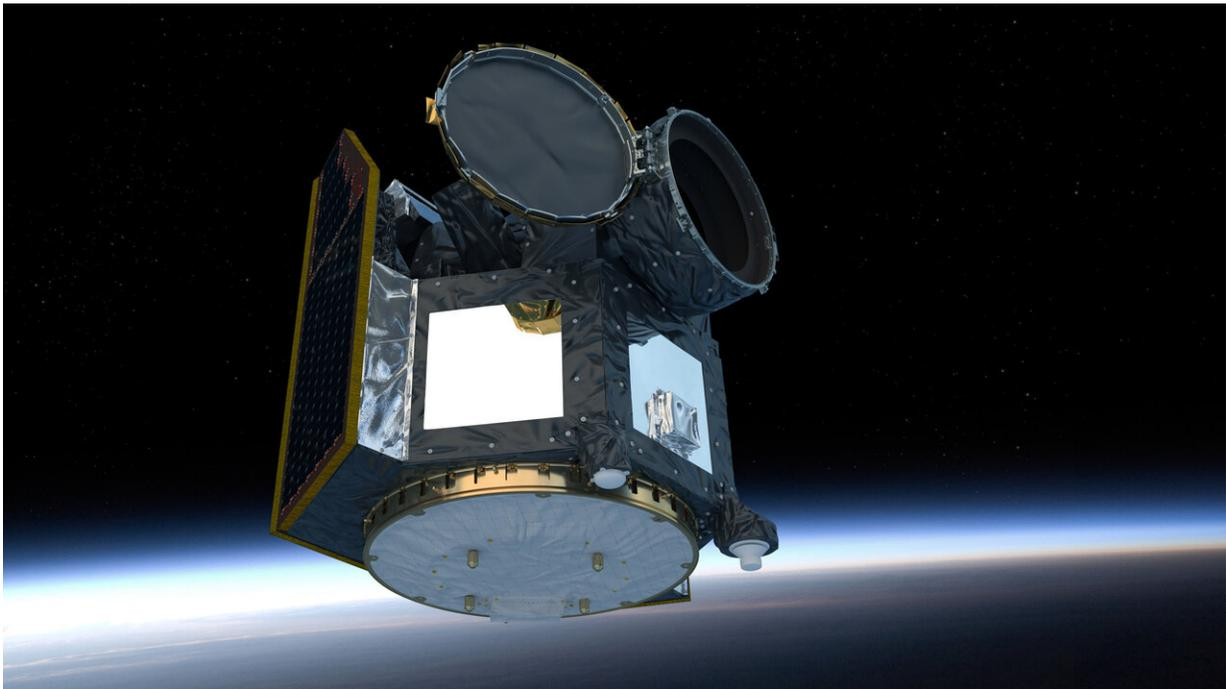
Artist's impression of Cheops, ESA's Characterising Exoplanet Satellite, in orbit above Earth. In this view the satellite's telescope cover is open. Credit: ESA / ATG medialab
