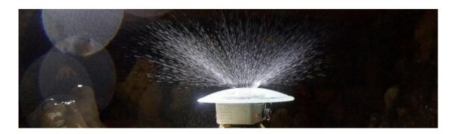
Dripping station at the Arcy-sur-Cure Cave (Yonne, Central-France). The dripping water is regularly sampled at this station and the modern calcite is gathered on a glass. Credit: D. Genty
