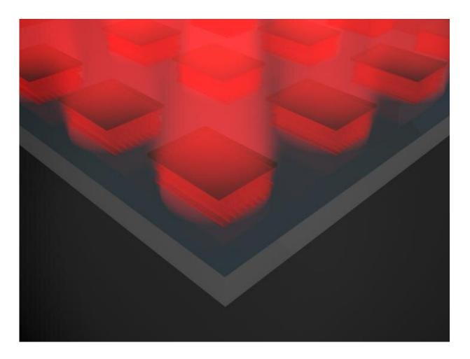
A Rice University simulation shows an array of cavities patterned into a film of aligned carbon nanotubes. When optimized, the film absorbs thermal photons and emits light in a narrow bandwidth that can be recycled as electricity. Credit: Chloe Doiron/Rice University
