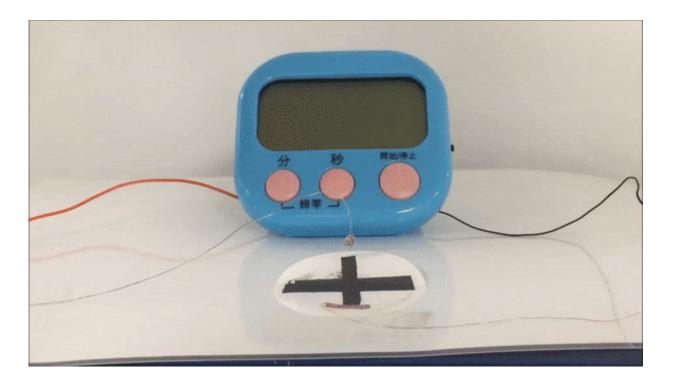
A real-time digital camera video of smart switch upon sequential on/off NIR light irradiation. Credit: Science Advances, doi: 10.1126/sciadv.aaw7956
