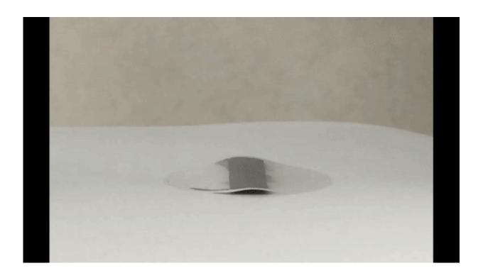
A real-time digital camera video of the MXCC/PC bilayer-structured actuator upon sequential on/off NIR light irradiation. Credit: Science Advances, doi: 10.1126/sciadv.aaw7956
