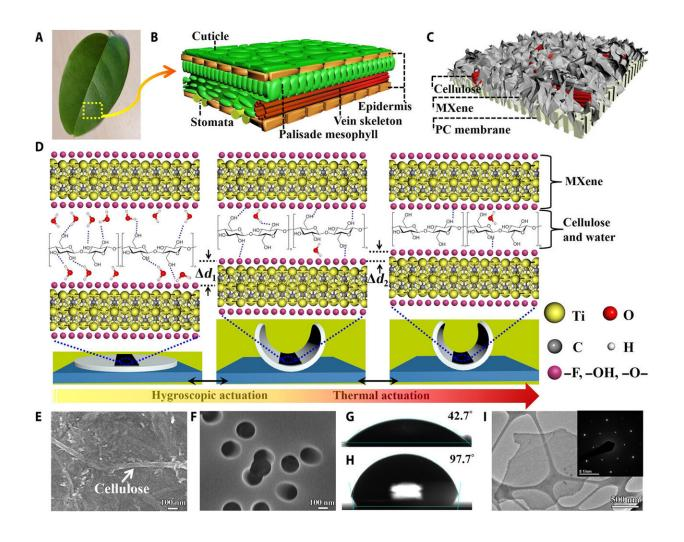
The elaborate structure, components, and actuation mechanism of the MXene-cellulose–based actuator. (A) Photograph of a natural leaf. (B) Schematic diagram of a leaf structure. (C) Schematic diagram of the MXCC/PC bilayer-structured actuator, which is composed of MXCC and a PC filter membrane. (D) Actuation mechanism of the MXCC/PC bilayer-structured actuator.
