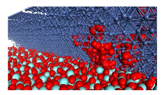
The initial positions of the atoms in this computer model of a solid-oxide fuel cell were based on observations of the actual atomic configuration using electron microscopy. Simulations using this model revealed a previously unreported reaction (red path) in which an oxygen molecule from the yttria-stabilized zirconia layer (layer of red and light blue balls) moves through the bulk nickel layer (dark blue balls) before forming OH on the nickel surface. Credit: Michihisa Koyama, Kyushu University
