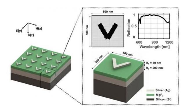
Schematic diagram of an artificial neural network that can design arbitrary photonic structures. Cross section of structures is mapped as two-dimensional cross-sectional bitmap so that artificial neural network can design structures of metasurface antenna which cannot be designed with structural parameters. Credit: POSTECH
