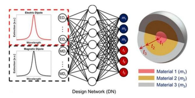
Schematics of and artificial neural network that can design structural parameters and material simultaneously. When desired optical properties (electric/magnetic dipole spectrum) is inputted, each thickness and types of materials of the three-layer core-shell nanoparticle are provided as output. Credit: POSTECH
