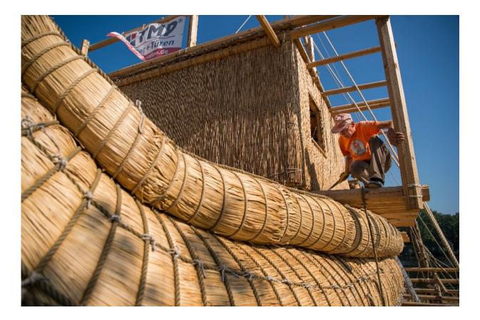
Large bundles of totora reed were lashed together with ropes to form the main body of the vessel before it was equipped with a wooden mast and two reed compartments for sleeping
