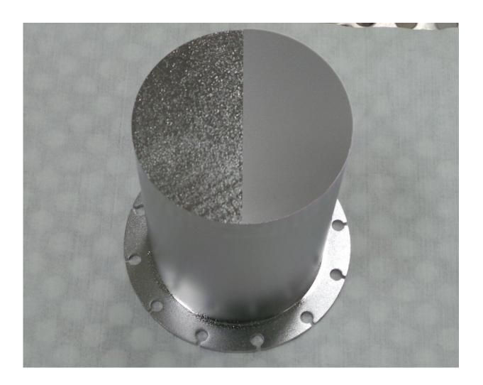
Photomontage shows a sample of solid, pure niobium before coating (left), and coated with a thin layer of Nb3Sn (right). Credit: HZB
