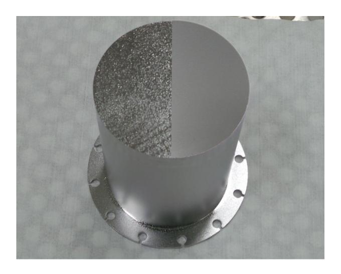
Photomontage shows a sample of solid, pure niobium before coating (left), and coated with a thin layer of Nb3Sn (right). Credit: HZB
