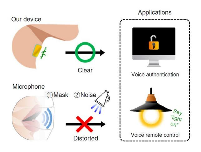
Schematic image of the comparison between our device and a reference microphone (Bruel & Kjaer, microphone type 4192, sensitivity of 1 V Pa?1) for voice authentication and voice-controlled applications. Credit: POSTECH
