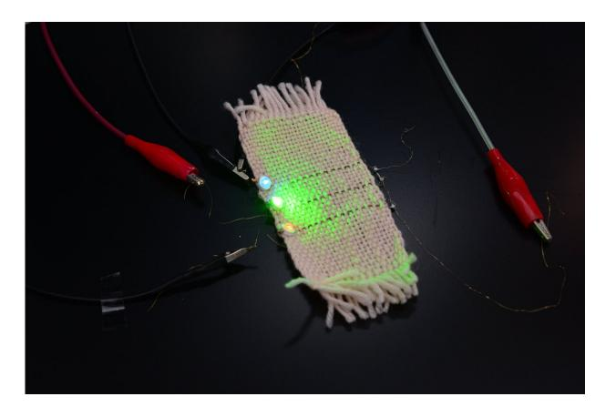
A new electronic textile developed by KIST's research team that turns on LEDs on top of fabric. Credit: Korea Institute of Science and Technology (KIST)
