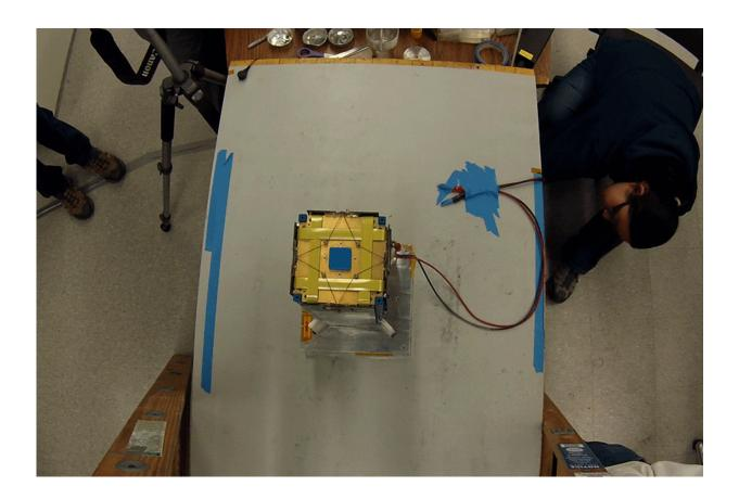
E-TBEx's deployment is tested at the Michigan Exploration Lab. Constructing and testing the E-TBEx CubeSats was particularly complex because of the multiple antennas and solar panels that deploy after launch. Credit: University of Michigan/Michigan Exploration Lab
