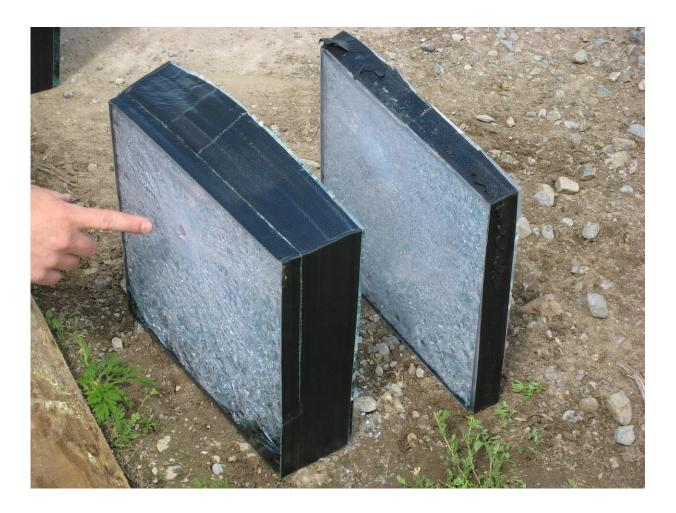
A projectile exit point is shown in the ballistic glass (left). The aluminum oxynitride transparent ceramic armor is shown (right) with a bulge and no exit from the projectile. Credit: Air Force Office of Scientific Research
