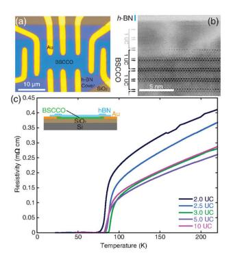
Graphic showing van der Waals BSCCO device. (a) Optical image of Hall bar device, (b) Cross-sectional view of a typical device in scanning TEM. Columns of atoms are visible as dark spots; black arrows point to bismuth oxide layers (darkest spots), while gray arrows show their extrapolated positions. (c) Resistivity as a function of temperature for devices of a different thickness. Credit: Argonne National Laboratory
