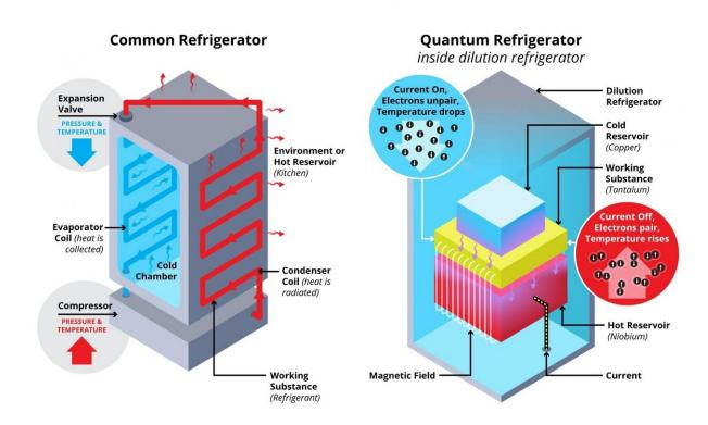
The superconductor fridge is similar to a conventional refrigerator, in that it moves a material between hot and cold reservoirs. However, instead of a refrigerant that changes from a liquid state to a gas, the electrons in a metal change from the paired superconducting state to an unpaired normal state. Credit: University of Rochester illustration / Michael Osadciw
