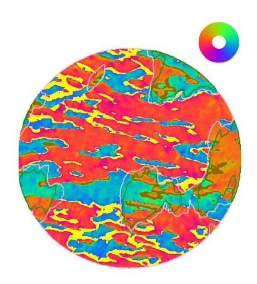
Magnetic vector map (50  $\mu$ m field of view) describing the magnetisation of a Ni film while applying 50 V across the ferroelectric substrate of PMN-PT. The colour wheel identifies magnetisation direction. Yellow and brown denotes
