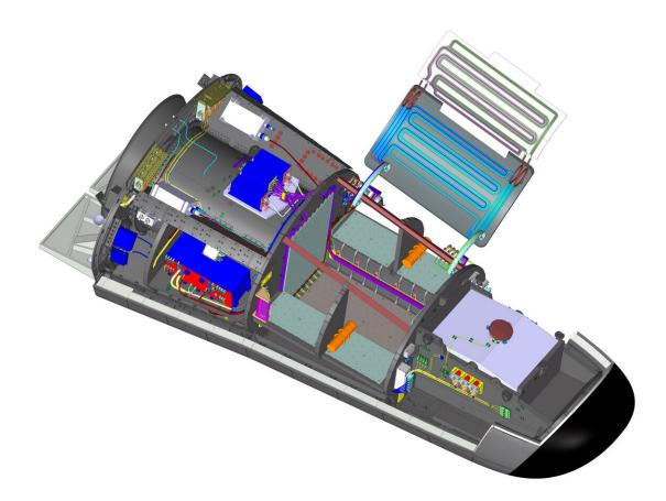
Up to 800 kg of payloads can fit inside Space Rider's environmentally controlled cargo bay that offers 1200 litres of payload volume and provides services including 600 watts of power along with thermal, control, data-handling and telemetry capability. Offering an array of orbit altitudes and inclinations, Space
