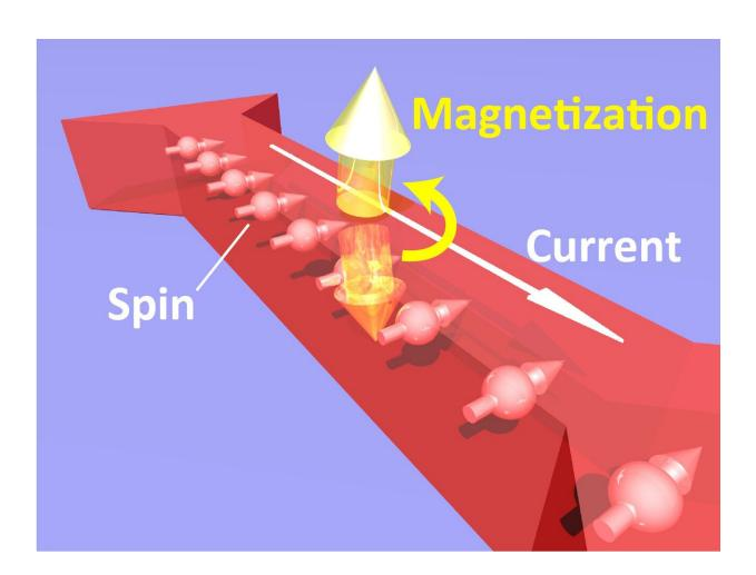
This diagram shows how magnetization reverses in a GaMnAs crystal. Credit: © 2019 Tanaka-Ohya Laboratory
