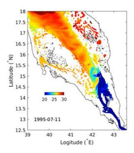
The Strait of Bab-el-Mandeb, as simulated by the KAUST model, shows the intrusion of the cold Gulf of Aden water into and out of the Red Sea in the summer at a depth of 80 meters. Credit: American Geophysical Union
