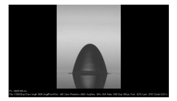
A water droplet, subject to an electric field of slowly increasing strength, suddenly bursts by emitting a fine, electrified mist from its apex. Credit: Massachusetts Institute of Technology
