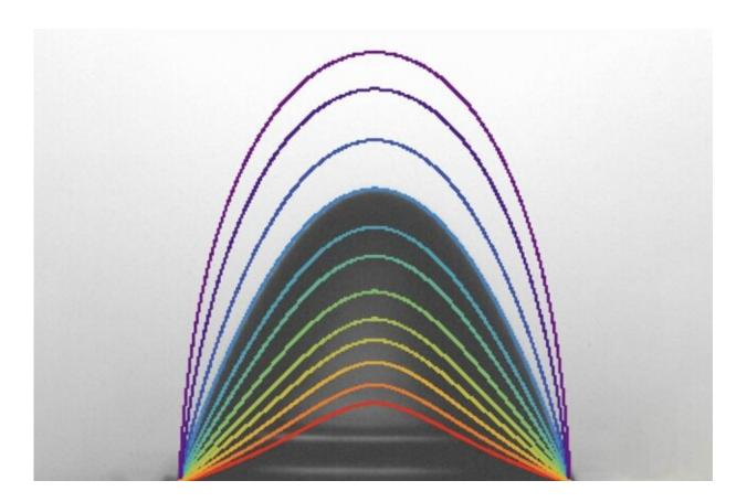
Electrified water droplets take on a variety of distorted shapes just before bursting, based on the strength of the electric field. The profiles of different distorted droplet shapes are shown, overlaid on an image of one particular distorted droplet for comparison. Credit: Massachusetts Institute of Technology
