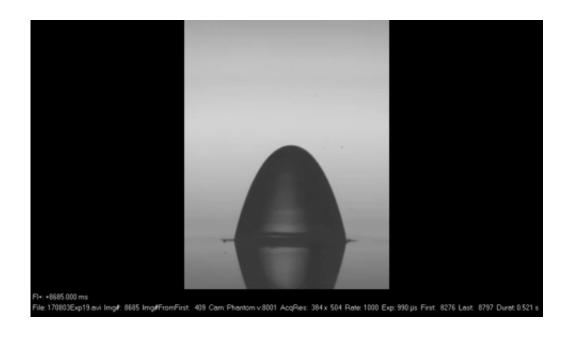
A water droplet, subject to an electric field of slowly increasing strength, suddenly bursts by emitting a fine, electrified mist from its apex. Credit: Massachusetts Institute of Technology
