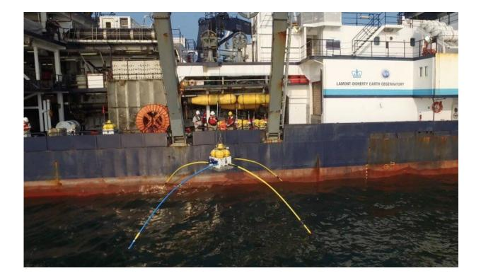
An electromagnetic receiver used in the study being deployed off the research
