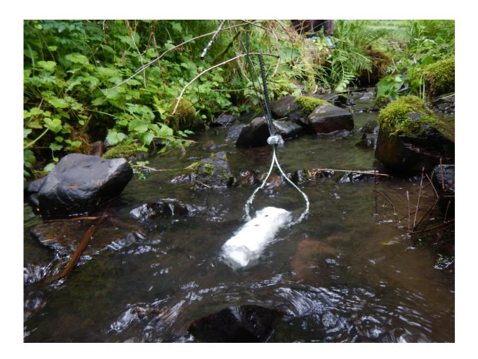
Researchers use thermistors in a PVC housing to monitor stream temperatures. Credit: Kevin Bladon
