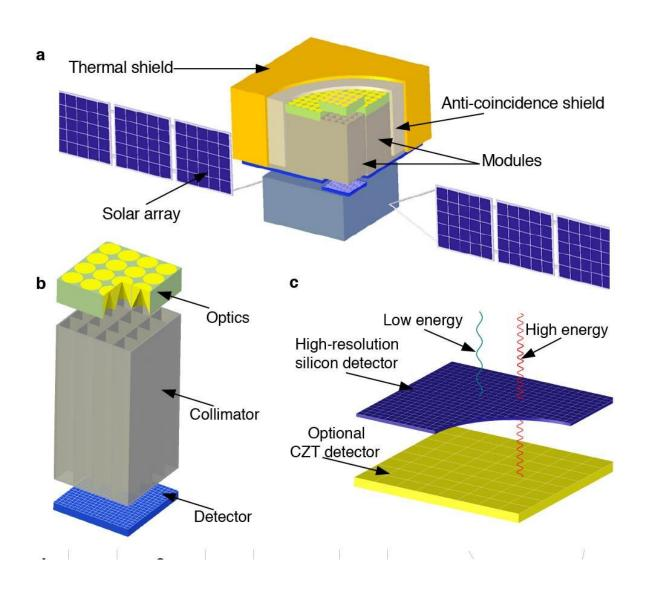
The design marks a radical departure from the so-called Wolter type space X-ray telescopes, which rely on mirrors to direct X-ray beams. Instead the proposed optics are built by stacking disks embedded with prismatic rings, created with
