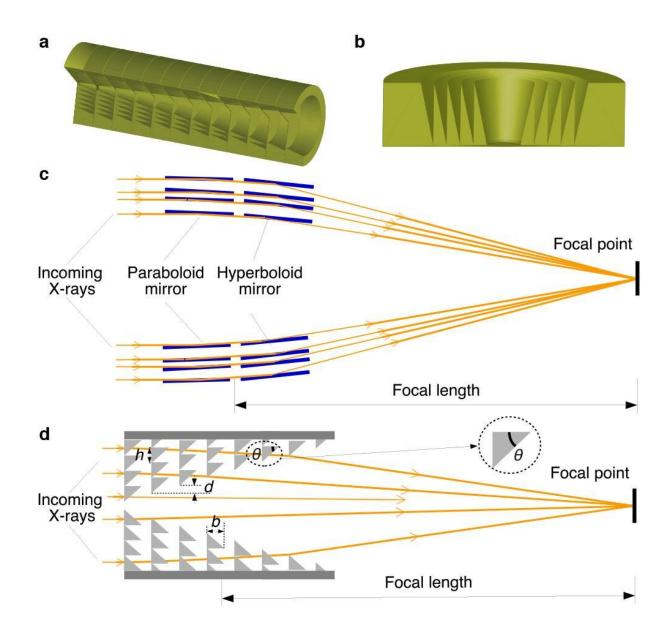
A cross section representation of how the new design differs from Wolter type X-ray telescopes. An assembly of disks with microengineered prisms guides the beam toward the focal point, rather than paraboloid and hyperboloid mirrors. Credit: Wujun Mi
