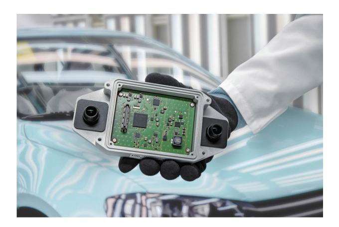
A shot of the camera/radar module with its housing. Credit: Fraunhofer-Gesellschaft
