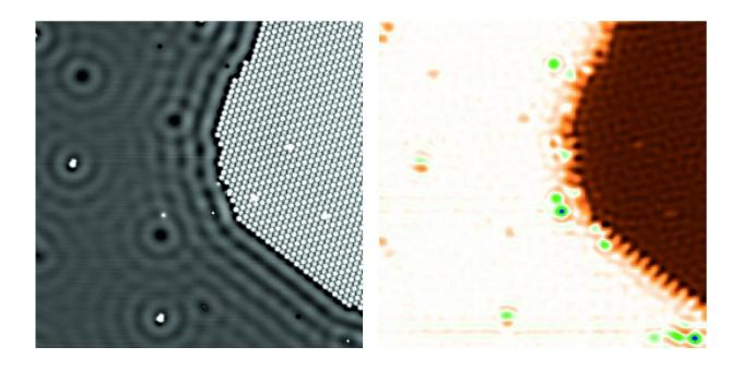
Image from a scanning tunnelling microscope (STM, left) and a scanning quantum dot microscope (SQDM, right). Using a scanning tunnelling microscope, the physical structure of a surface can be measured on the atomic level. Quantum dot microscopy can visualize the electric potentials on the surface at a similar level of detail -- a perfect combination. Credit: Forschungszentrum Jülich / Christian Wagner
