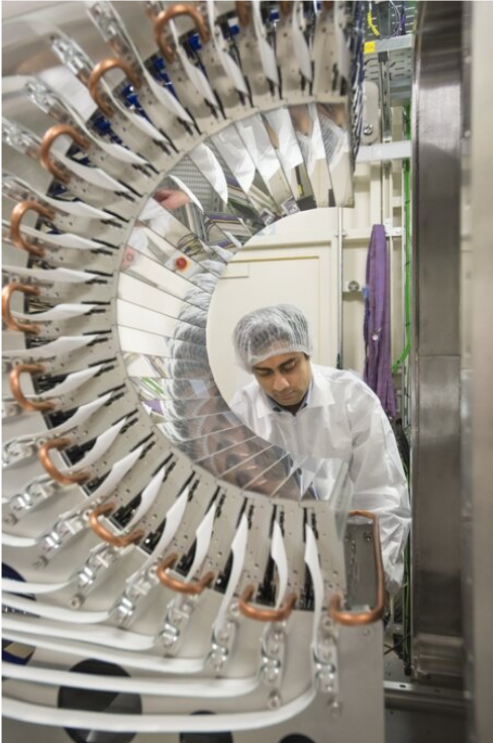
Vinay Grama, I23 beamline project engineer with the PILATUS 12M detector during installation. Credit: Diamond Light Source
