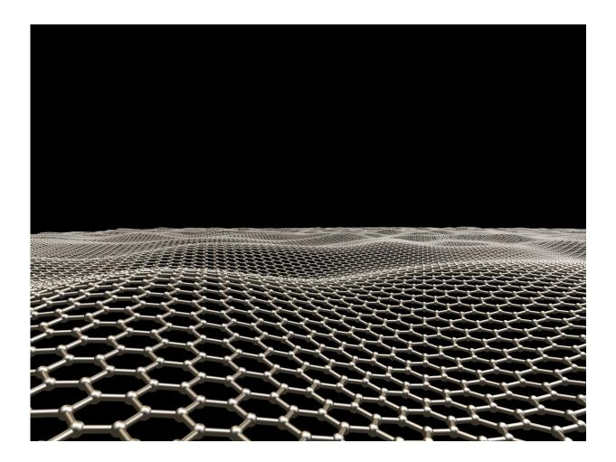
Graphene is made of carbon and is the thinnest material in the universe, only one atom thick. Credit: University of Oklahoma
