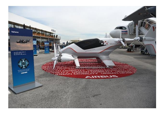
The Vahana is Airbus's single-seat prototype all-electric, tilt-wing aircraft to
