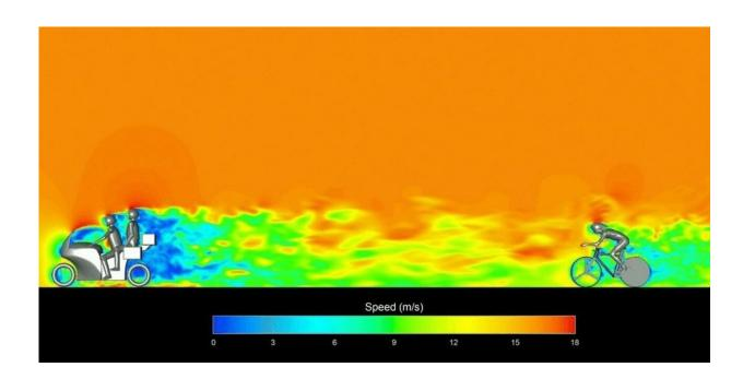
Computer simulation of a rider cycling at a distance of 10 meters from a motorcyclist. The green and yellow colors in front of the rider show that the airspeed here is substantially lower than in front of the motorcycle. Credit: Bert Blocken
