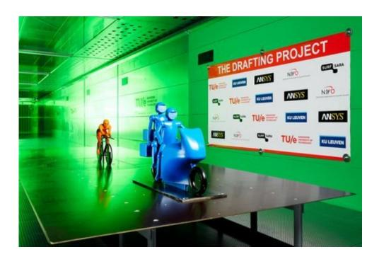
Experiment with a rider cycling behind a motorcycle in the wind tunnel of Eindhoven University of Technology. Credit: Bart van Overbeeke
