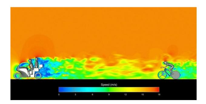
Computer simulation of a rider cycling at a distance of 10 meters from a motorcyclist. The green and yellow colors in front of the rider show that the airspeed here is substantially lower than in front of the motorcycle. Credit: Bert Blocken
